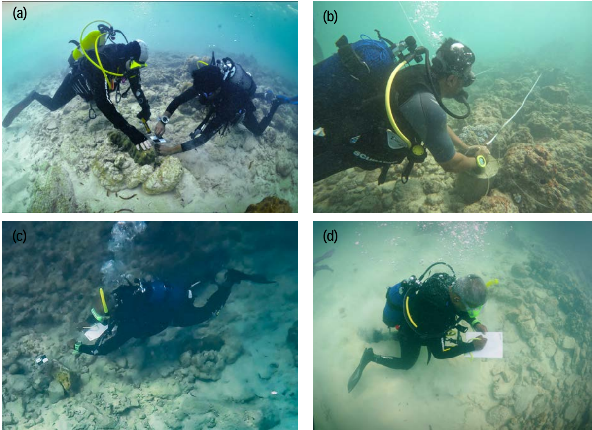
Figure 8: 3D trilateration operations: (a) setting markers; (b) measuring distance between markers; (c) measuring depth of the markers; (d) recording the measurements.
