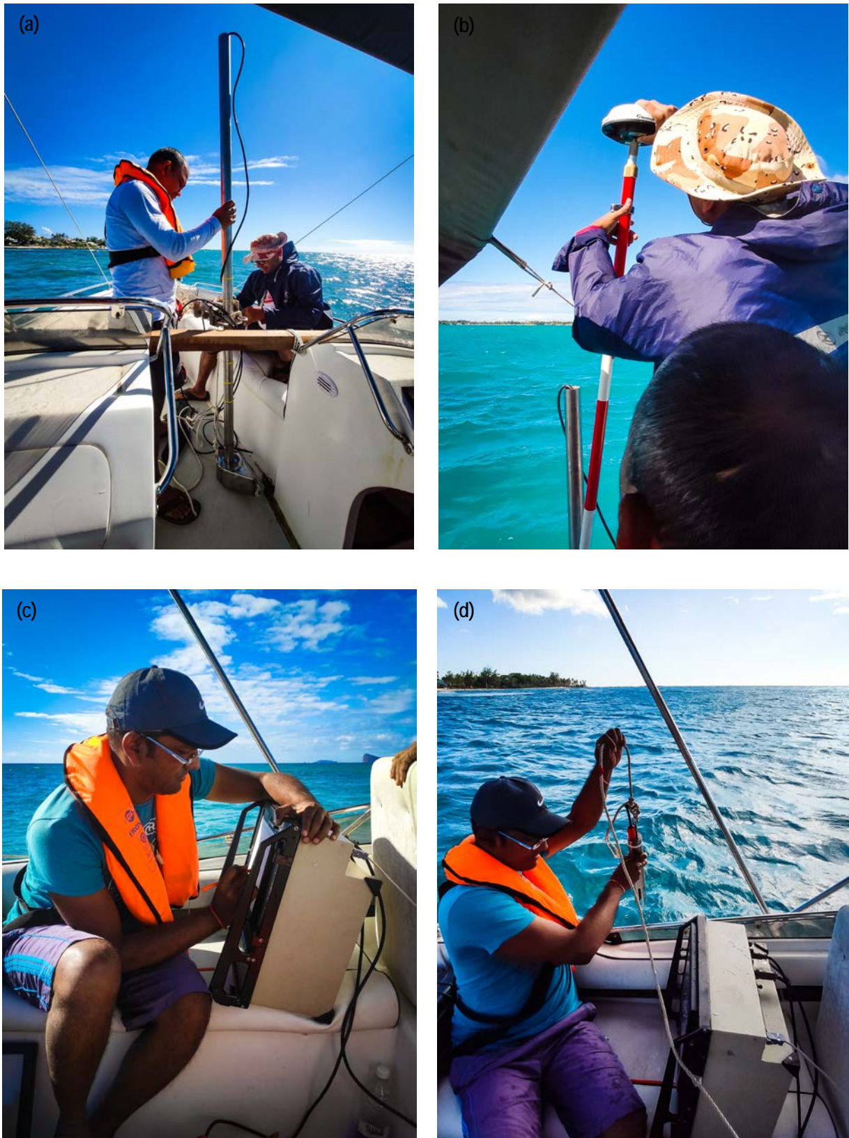
Figure 4: (a) Setting up the SBES transducer; (b) the GPS antenna and SBES transducer mounted in-line vertically; (c) the SBES logging system; (d) Casting CTD to observe the Sound Velocity Profile.
